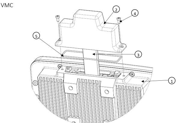
Attention before assembling please check the height of the USB stick and the depth of the Top Cover for LTE WWAN USB & Dual Antennas. The height of the USB stick must be smaller than the depth of the Top Cover for LTE WWAN USB & Dual Antennas.
